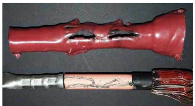
Fig.3: Cable termination insulation failure due to electrical surface tracking [16].
